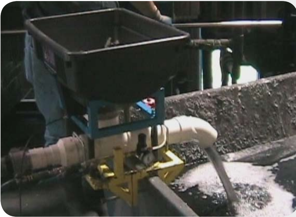
Latex flowing through LiquiSorb feeder mounted to dump cart
