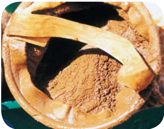
Iron solids in a sock filter during the initial treatment process. CETCO incorporated a process to remove the iron from the stream.
