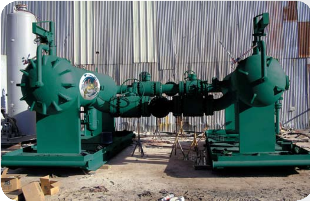
Pipeline Dual FilterSep
