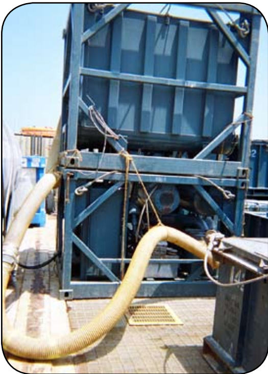
Hands-free transfer of solids to shipment/ storage tank
